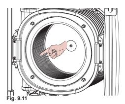
If the condensate primary exchanger elements are dirty (notable only after removing the burner body), brush them using a bristle brush and remove the dirt using a suction device.
